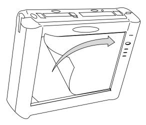
Figure 4. Removing the Protective Film
